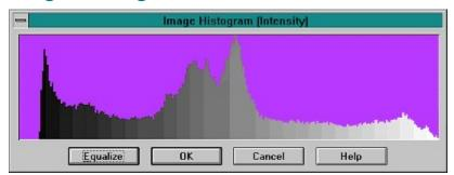
This option displays a histogram of the intensity of the image. It shows the relative number of pixels at each intensity level. If the values are bunched together, the picture lacks contrast; if they are skewed to the left or right, the picture is most likely too dark or too light.
